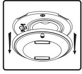
7. Remove paint mask unless painting is required. In that case, follow steps 8-11 when painting is complete.
